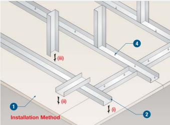
Construction of ceiling showing ceiling channel section fixing.
