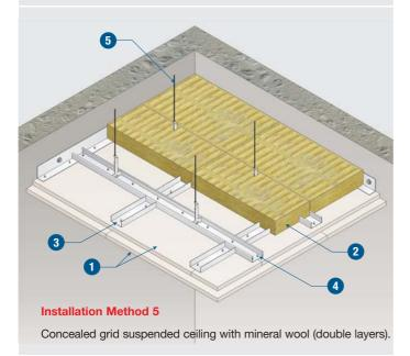
All systems detailed within this page allow for the protection to, or from, services contained within the ceiling void. These systems will also provide protection to steel beams in accordance with the criteria of BS 476: Part 23: 1987 where exposure to fire is from below.
