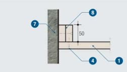
Detail 3 Alternative wall connection (Section A-A)
