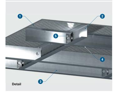
PROMATECT®-S ceilings provide horizontal barriers against fire tested and approved in accordance with the relevant criteria of BS 476: Part 22.
