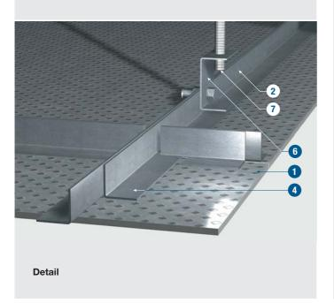
PROMATECT®-S ceilings can also be fabricated using angles inlieu of channels. The angles are bolted or welded back to back to form a T-section.
