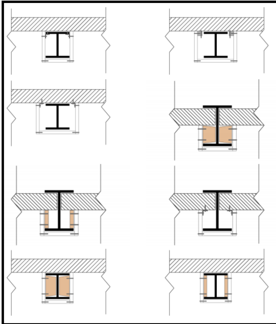
Figure 8 - Three Sided Beam Encasements
