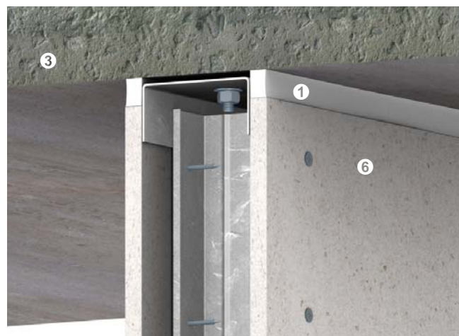
Typical head and control joints of lightweight partition (STC 39)
