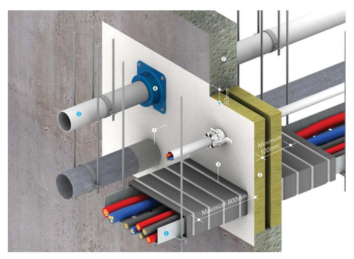
Up to -/180/180 fire resistance in accordance with the requirements of BS 476: Part 20: 1987, BS EN 1366: Part 3: 2009 and/ or AS 1530: Part 4: 2014, depending on applications and types of penetrating elements; insulation time is the measured time to insulation failure on surface of the PROMASEAL® Bulkhead Sealer
