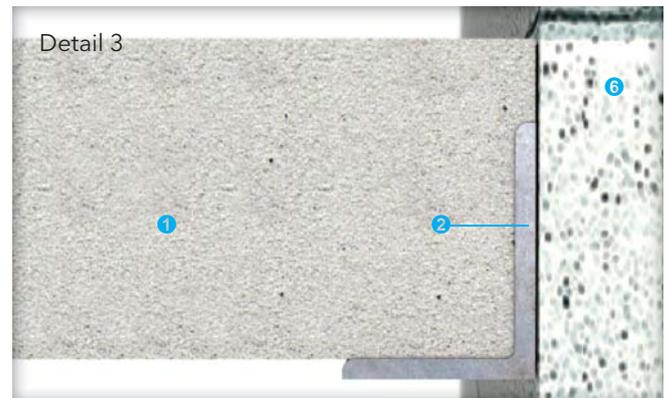
Up to -/240/240 fire resistance in accordance with the requirements of BS 476: Part 20: 1987, BS EN 1366: Part 3: 2009 and/or AS 1530: Part 4: 2014, depending on applications and types of penetrating elements; insulation time is the measured time to insulation failure on surface of the PROMASEAL® Mortar
